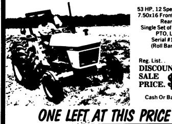
53 HP, 12 Speed Syncro Shift, 7.50x16 Front Tires, 16.9x30 Rear Tires. gle Set of Remotes, 540 PTO, Live PTO Serial #11056389 (Roll Bar Optional)
