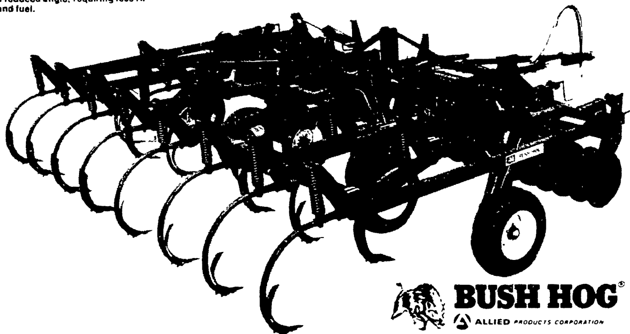
Rigid shanks are recommended for use in soils free of rocks and stumps. Shear pin protection is standard equipment. Shanks contact the soil at a reduced angle, requiring less HP and fuel.
