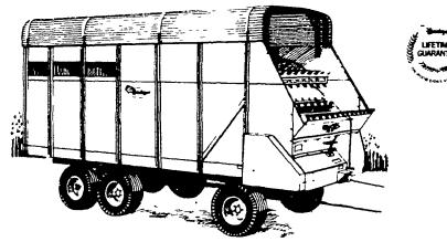
Start with specially treated acid resistant exterior grade plywood, bolted to steel channel stakes. No nails anywhere. Add to that a tough welded and bolted undercarriage built to carry the big loads. Match all this with Badger's simple and reliable heavy roller chain drive, a beater design . that delivers a smooth even discharge to the blower. And then mount it on Badger's own heavy duty single or tandem axle running gear and you've got a box that will stand up to the toughest punishment.
