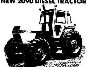
With Mechanical Front Wheel Drive, 16.9x28 Front Tires, 20.8x30 Rear Tires, On The Go Power Shift Transmission, Cab. Air, Heat
