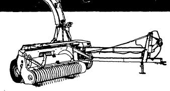
The Model 782 is built for heavy-duty performance. The 12-knife cutterhead chops uniformly, without a recutter screen. But for special crops and conditions, recutter screens are available. Check these outstanding features.
