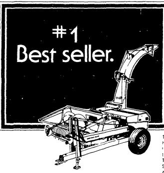
The country's best selling medium-duty forage harvester is the Model 718 from Sperry New Holland You get a fine, uniform cut with low power requirements. Exclusive underbeveled knives eliminate rebeveling and make knife sharpening fast and easy. Flip-up feedroll makes shearbar adjustment easy. Twelve-knife cutterhead has reversible, double edged knives. You can choose from one or two row low profile crop heads, windrow pickup or sicklebar.
