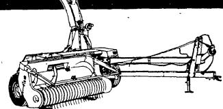
The Model 782 is built for heavy-duty performance. The 19-knife cutterhead chops uniformly, without a recutter screen. But for special crops and conditions, recutter screens are available. Check these outstanding features.
