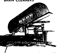
Berg Gutter Chain is a series of one piece links hooked end to end, which makes it easy to remove links and eliminates the need for all those pins rivets and boits. The heavy concentration of metal in the hooks and at the pull points gives the Berg Chain Link more pull strength than ordinary links The links are 71/2 inches long, 21/4 inches wide and 1/2 inch thick and weigh over two pounds Each link is forged from special alloy forging steel in a single piece No worry about corrosion
