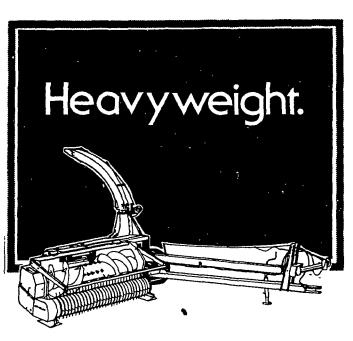
The Model 892 is the biggest capacity pull-type forage harvester offered by Sperry New Holland Built for bigtractor horsepower, the "892" can be used with tractors up to 175 horsepower
