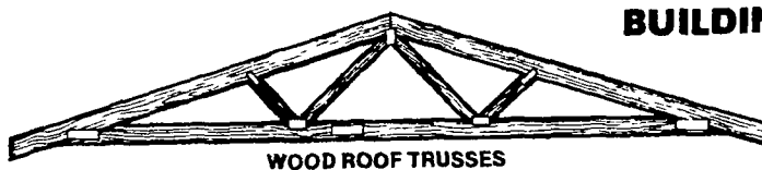
WOOD ROOF TRUSSES
