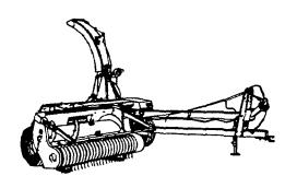
The Model 782 is built for heavy-duty-performance. The 12-knife cutterhead chops uniformly, without a recutter screen But for special crops and conditions, recutter screens are available. Check these outstanding features:
