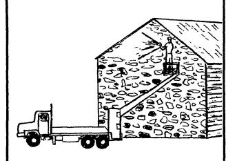
REPAIRING STONE WALLS with SPRAYED ON PRESSURE CONCRETE
