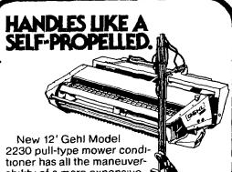
ability of a more expensive self-propelled Hydraulic center-pivot Swing-Frame assembly lets you pull from the right or left side of your tractor All hydraulic drive keeps you moving smoothly, and the big 20" auger moves the crop into 57" conditioning rolls for pre-
