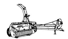
The Model 892 is the biggest capacity pull-type forage harvester offered by Sperry New Holland Built for big tractor horsepower, the "892" can be used with tractors up to 175 horsepower
