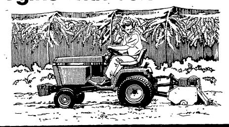
spider, can also be set for standard rotation. The gear-type transmission has 4 forward speeds, plus reverse.
