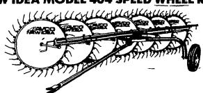
The 404 Wheel Rake is a high quality rake at a reasonable price. Rakes fast and clean in any field... smooth, uneven, contoured or hilly. Plus, it costs less to buy and less to maintain.
