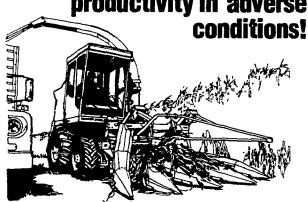
Hesston/Field Queen SP Forage Harvesters all feature power-efficient 6-knife cutting cylinders. Six-knife design gives more room between knives, so more crop gets in, giving you more capacity.
