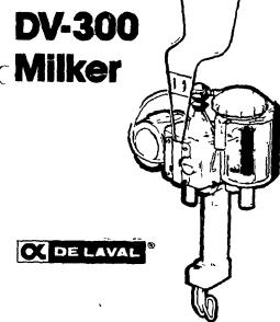
The De Laval® DV-300™ milking system senses milk flow and automatically shifts vacuum levels and pulsation rates for stimulation, milking and post milking. That means less stress on your cows and improved milking routine for you. The DV-300 milker...the flow controlled milking machine that brings affordable semi-automated nilking to all types of dairy operations. See us for full information on the DV-300 milker and the full line of De Laval dairy equipment, all
