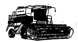
SPERRY NEW HOLLAND TWIN ROTOR COMBINES GIVE YOU A PATENTED DUAL ROTOR THRESHING PROCESS WHICH PRODUCES A CLEANER SAMPLE, WITH LESS GRAIN DAMAGE AND LOWER LOSSES.
