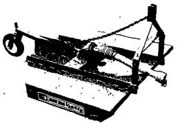
· Flexible linkage allows smooth cutting on uneven terrain. ASAE Cateogry 3 universal joint is standard equipment
