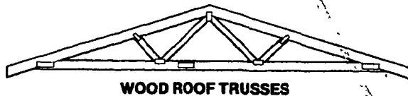
WOOD ROOF TRUSSES
