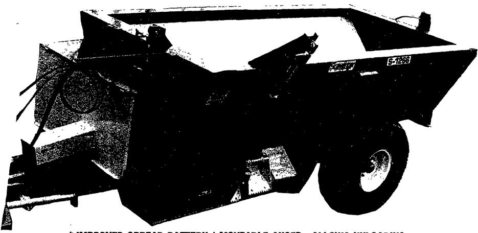
\* IMPROVED SPREAD PATTERN \* MOVEABLE AUGER - ALLOWS UNLOADING EVEN THE TOUGHEST MANURE \* HI-DENSITY POLYMER LINER - PREVENTS FREEZING IN WINTER \* 1150 GALLONS \* ONLY 63" HIGH • OPERATES ON ONLY 60 H.P. \* 222 BU. HEAPED (OTHER SIZES AVAIL. TO 386 BUSHELS.)
