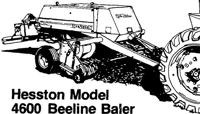
Hydraulic-driven bale thrower (optional) saves time and labor.
