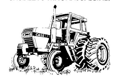
128 hp (95kW) Tractor with Cab & Air, has long life 504-cu. Casebuilt diesel engine; all new hydraulics; big quiet cab and dozens of features for your comfort and field productivity!
