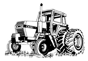
128 hp (95kW) Tractor has long life 504-cu. Case-built diesel engine; all new hydraulics; big quiet cab and dozens of features for your comfort and field productivity!
