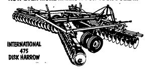
17 Ft. Folding Wings, 9.5L Flotation Tires, Heavy Duty Disk Blades, Cylinder & Hoses, Furrow Fillers
