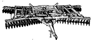
Positive depth control is incorporated into the hydraulic axle control to assure uniform cutting depth. It eliminates the guesswork, and the adjustment is easy
