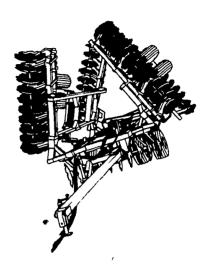
The tandem models feature a center mounted, self-cleaning knife to break the center ridge for complete soil-leveling action
