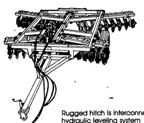
Notched or plain blades are available on all tandem models. All offset models are available with notched blades. Some offset models offer a choice of notched or plain blades. Rear sections on both tandem and offset models feature a stepped-down blade configuration for optimum soil leveling action.
