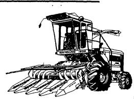
The 250-hp Model 1900 chopper features an exclusive electronic metal detector that reduces harvester damage, and helps cut down on hardware disease. Exclusive underbeveled knives never need rebeveling. Exclusive flip-up feedrolls make shearbar adjustment easy. Exclusive interchangeable cropheads - ideal for the farmer/rancher who chops both windrowed crops and row crops. Plus a big choice of other crop heads. Under-knife baffles increase capacity.
