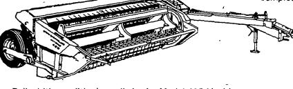
Full-width conditioning rolls in the Model 489 Haybine" mowerconditioner are located in the main frame, not the header. The lighter header responds quicker to ground contours and greatly reduces knife and guard damage. The "489" is designed for operators who demand the very best.
