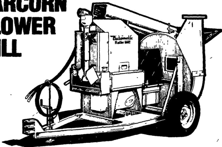
Automatic pioneered the development of the unique crusher unit which shells corn and shreds the cob ahead of the rollers which crack the kernels and reduce the cob further. No troublesome screens to change or slow down the capacity. It comes with 8-foot hydraulic intake auger and 54-inch blower. Also available with an 11-inch tilting discharge auger with 10-foot reach in place of the blower.
