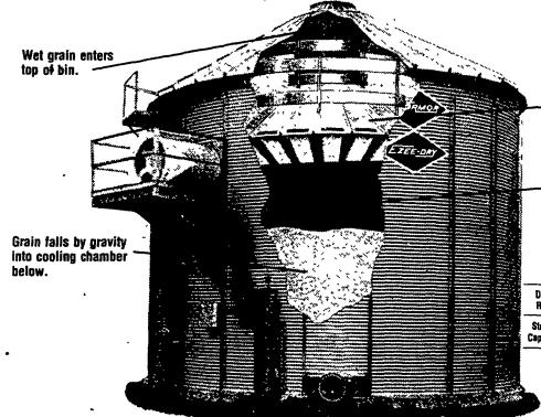
Grain is dried in overhead drying floor through thin grain column.
