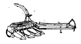
The Model 892 is the biggest capacity pull-type forage harvester offered by Sperry New Holland Built for big tractor horsepower, the "892" will power through the driveline, and be used with tractors up to 175 horsepower.
