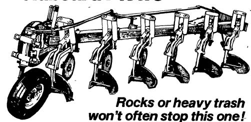
You can't beat 'em for heavy duty nonstop plowing in your toughest fields. With exceptional vertical clearance and automatic reset trip beams, 720 plows take heavy trash and hidden obstructions in stride. Also ideal for minimum tillage and soil conservation practices because of great trash clearance and wide-slab furrows-especially with the big 20-in. size-often eliminating an extra operation of disking crop residues before plowing. Also Finance plans available.
