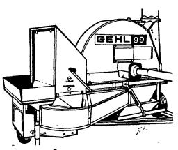
The Gehl 99 forage blower ends silo bottlenecks. Two hopper feed tables throw material into the fan for a fast start. And 12 staggered blades, six on each side of the blower fan, move silage to the top in a hurry. Stop in and talk to us today.
