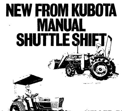
Now you can change from forward to reverse without touching the gearshift. Simply disengage the clutch, stop the tractor, and pull the shuttle lever down in one straight non-stop motion.
