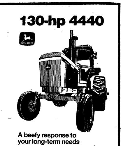
The 4440 is indeed a powerful performer. But just as important, it has the strength to back up that power in the field. From stem to stern, it's beefier than its predecessor. There's a bigger-displacement engine, new engine cooling system, bigger transmission/hydraulic oil cooling system, multi-pinion differential, wider final drives, and bigger drive axles. These are just a few of the points we'd like to cover when you stop by the store and ask for more information on the 4440.
