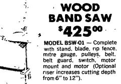
Capacity: depth of throat 10"; cut 6", \*12" with optional riser kit Model R6, blade width (max.) 3/8"; length 72"; adjustment 711/2"/721/2". Table: working surface 10"Wx10"D, tilt 45°R/5°L; height from floor 411/2". Speed (SFM) 2400. Bearings: upper wheel (1), lubricated, bronze; lower wheel (2) lubricated bronze Motor (standard) 1/2 HP. Overall size 20"W x 13"D x 501/2" H; Shipping weight (approx.) 115 lbs
