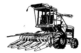
The 250-hp Model 1900 chopper features an exclusive electronic metal detector that reduces harvester damage, and helps cut down on hardware disease. Exclusive underbeveled knives never need rebeveling. Exclusive flip-up feedrolls make shearbar adjustment easy. Exclusive interchangeable cropheads — ideal for the farmer/rancher who chops both windrowed crops and row crops. Plus a big choice of other crop heads. Under-knife baffles increase capacity.
