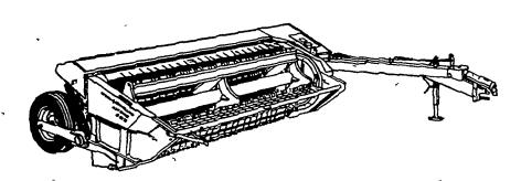
Full-width conditioning rolls in the Model 489 Haybine® mower-conditioner are located in the main frame, not the header. The lighter header responds quicker to ground contours and greatly reduces knife and guard damage. The "489" is designed for operators who demand the very best.
