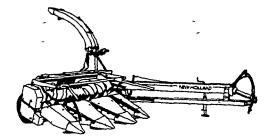
There's a big choice of crop heads, including the exclusive interchangeable 3-row crop head/windrow pickup, 2-row low-profile crop head; conventional windrow pickup, sicklebar and ear-corn snapping heads. Under-knife baffles increase capacity.
