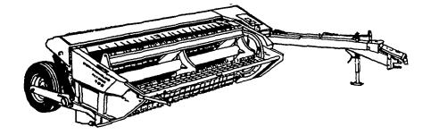
Full-width conditioning rolls in the Model 489 Haybine<sup>®</sup> mowerconditioner are located in the main frame, not the header. The lighter header responds quicker to ground contours and greatly reduces knife and guard damage. The "489" is designed for operators who demand the very best.
