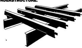
Two full length longitudinal sills of formed steel on regular duty models and structural steel on heavy duty models are reinforced on both sides, front and rear, with multiple steel gussets for extra strength and rigidity Longitudinals and heavy gauge steel full width cross sills are interlocked and electrically welded to the tough side rails and sills. Extra cross members in front of and behind the wheel pocket add extra load support
