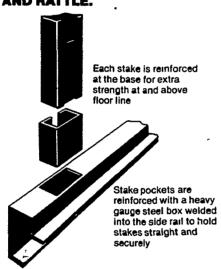
**REINFORCED STEEL GIRDER** UNDERSTRUCTURE.
