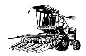
The 250-hp Model 1900 chopper features an exclusive electronic metal detector that reduces harvester damage, and helps cut down on hardware disease. Exclusive underbeveled knives never need rebeveling. Exclusive flip-up feedrolls make shearbar adjustment easy. Exclusive interchangeable cropheads — ideal for the farmer/rancher who chops both windrowed crops and row crops. Plus a big choice of other crop heads. Under-knife baffles increase capacity. complete stock of hay tools
