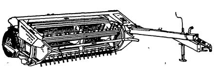
Full-width conditioning rolls in the Model 474 Haybine® mower-conditioner are located in the main frame, not in the header. The lighter header responds quicker to ground contours and greatly reduces knife and guard damage. Come in and let us demonstrate this deluxe machine for you.
