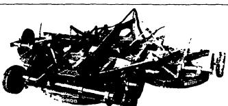
15' of flexible muscle with three sets of overlapping blades for complete cut. A
