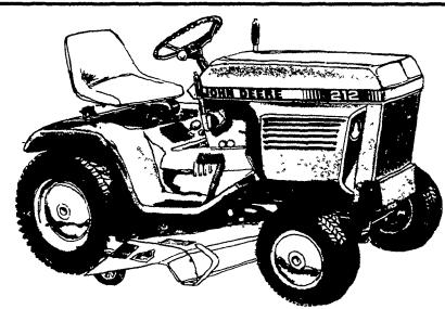
All feature an adjustable high-backed seat, roomy operator's area, and a fully enclosed engine for comfortable, quiet operation. For safety, there's a triple-safety starting system to guard against accidential starts. Easy-toidentify color-coded controls. And a switch that automatically shuts off the engine if you leave the seat with the PTO engaged.
