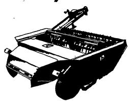
Crooked fence lines, uneven terrain, steep hillsides — they can steal your haying efficiency. Tackle them with our 1207 Mower/Conditioner — the compact machine with big-capacity features. Adjustable roll pressure, platform float, platform stabilizer, flotation tires tucked close to cutterbar, side-to-side and front-to-back balance...all combine to conquer small, irregular fields.
