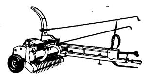
The 3940's power-efficient design begins with our Dura-Drum<sup>TM</sup> cutterhead...uneven forage doesn't stand a chance against its 36 segmented knives. And if a knife gets damaged, you'll find it's easy and inexpensive to replace one of the short blades.
