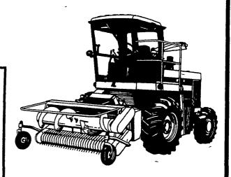
Now there are self-propelled forage harvesters that will give you increased productivity and the clean, uniform cut you want. The new 5720 and 5820 Self-Propelleds from John Deere. Their time-saving design starts with the Dura-Drum<sup>TM</sup> cutterhead...40 segmented knives on a 24-inch-diameter cutterhead cut through thick crop mat hundreds of times every second.
