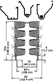
Manure is deposited on rust proof fiber glass manure chutes under each tier of cages and removed automatically by a Diamond manure removal system
