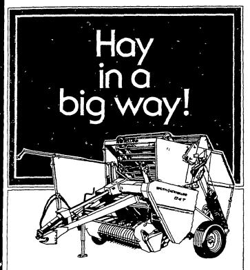
The Model 847 round baler makes bales weighing up to 850 pounds. You have three tying choices—manual, hydraulic and Auto-Wrap. And you'll get sure, fast core formation. Super-Sweep pickup and fines saver pans get more hay in every bale. See how easy it is to put up tons of hay in a day with a Sperry New Holland round baler. Ask us for a demonstration.
