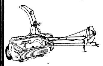
The Model 782 is built for heavy-duty performance. The 12-knife cutterhead chops uniformly, without a recutter screen. But for special crops and conditions, recutter screens are available. Check these outstanding features:
