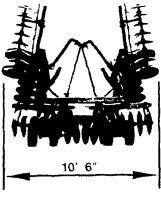
degrees They fold totally within the 106 cutting width of the center section (Most competative units have transport widths in excess of 14' With wings folded this harrow can easily pass through a 11' gate (This applies to all model variations of the Flex 90)
