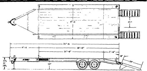
MODEL-86DOW Weight 4200# Capacity - 12000 # @60 mph, Overall Length - 24'6", Overall Width - 96", Bed Length - 18'0" Bed Width 96" Bed Height - 34" TIRES 9 50x16 5 10 PR / 8 Hold Budd' Wheels BRAKES Electric 12x2, one on each wheel Truck kit includes controller and complete wiring TOW HITCH Adjustable for 3 heights DECK 2" hardwood - installed lengthwise COLOR Highway Yellow RUNNING GEAR Multiflex Design LIGHTS & ELECTRIC SYSTEM Complete Set Furnished 12 Volt
