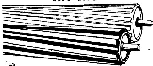
Big conditioner rolls adjust for gentle or aggressive action
