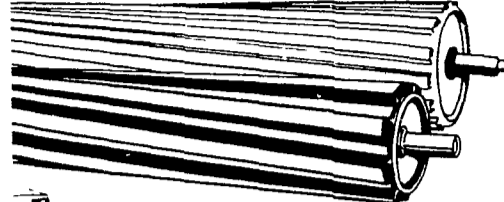
Big conditioner rolls adjust for gentle or aggressive action
